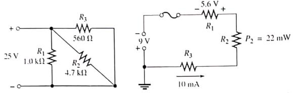
Q#02: Find the voltage at the indicated points in the figure given below. Assume the ground is connected at point C. (5)
